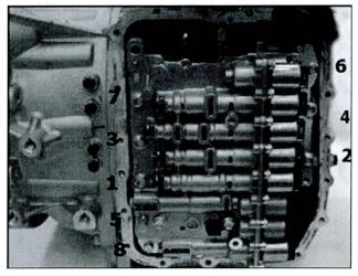
23. Reconnect the solenoid harness to the solenoids and oil temperature sensor.
