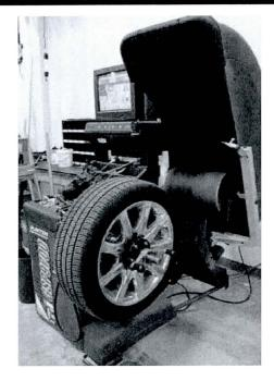
6. Remove all weights and re-balance all assemblies with any imbalance detected.
