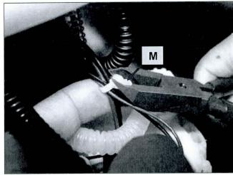
b. Disconnect the fuel pump and sender connectors. (N)
