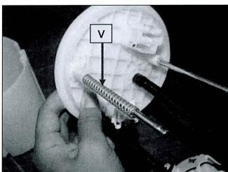
i. Install the removed spring (V) to the new plate until a "click" sound is heard.
