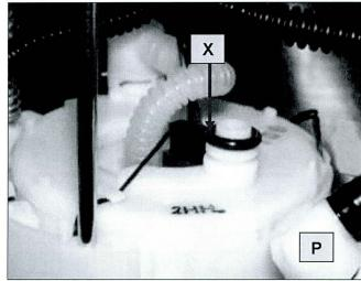
Connect the top plate pipe fitting (P) to the fuel filter outlet port and then install a new clip (Y) to secure it.
