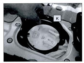
h. Remove the fuel pump module (L).
