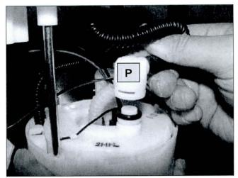
e. Undo the locks (Q) of the fuel pump plate stanchions, and then remove the fuel pump plate from the fuel pump module.
