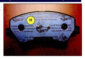
9. Install new brake inner and outer pad.
