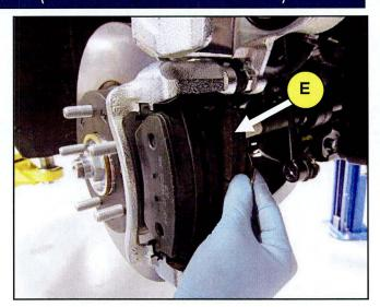
7. Remove the brake outer pad (F).
