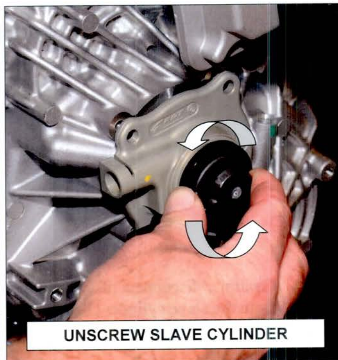
Figure 19 – Hold the Slave Cylinder Rod while Unscrewing the Clutch Slave Cylinder Assembly from the Slave Cylinder Rod
