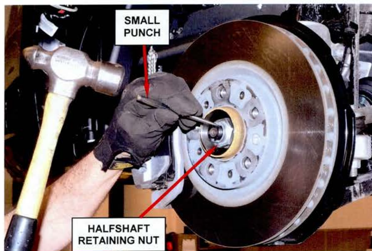
Figure 6 – Open Crimps on Halfshaft Retaining Nut
