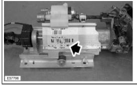
6. Insert the special tool (QME500100) into the square drive of the spindle.
