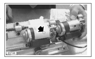
15. CAUTION: Insufficient application of grease can lead to the noise returning.
