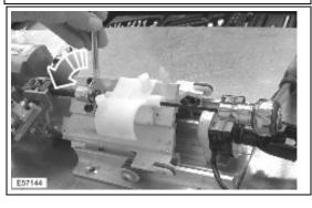
8. While holding the shaft with the tool, tighten the spindle nut to 6Nm.
