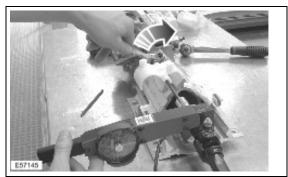
9. While holding the shaft with the tool, release the spindle nut one flat.
