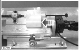
7. While holding the shaft with the tool, release the spindle nut half a turn.
