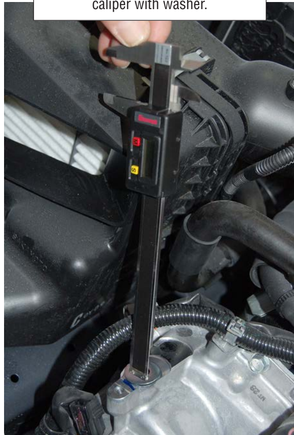
Measurement taken using digital caliper with washer.
