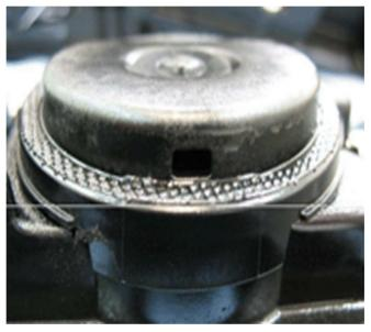
**Note:** The old style camshaft cover has a taller design PCV cap as shown in the illustration above.
