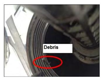
• Clean debris from oil filter housing and reinstall.
