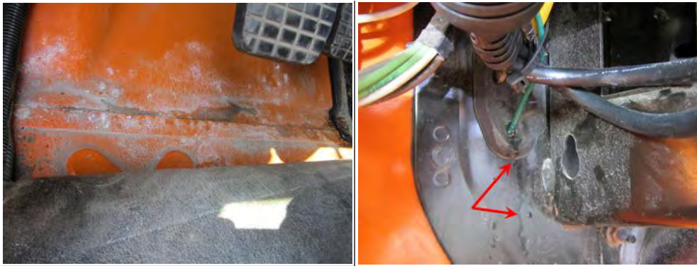
*Evidence of the leaks on older trucks*
