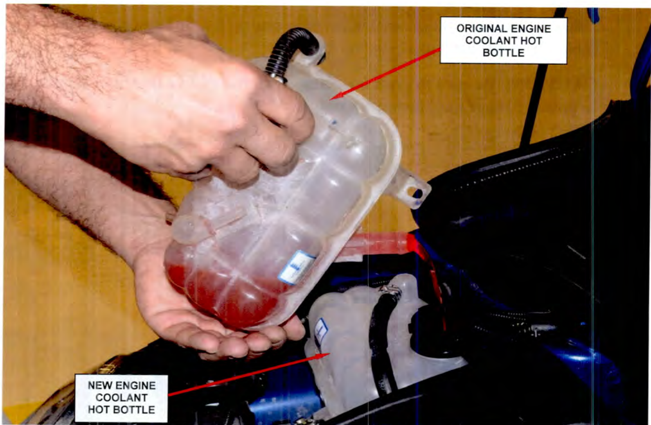
Figure 5 – Transfer Coolant from the Original Engine Coolant Hot Bottle to the New Engine Coolant Hot Bottle
