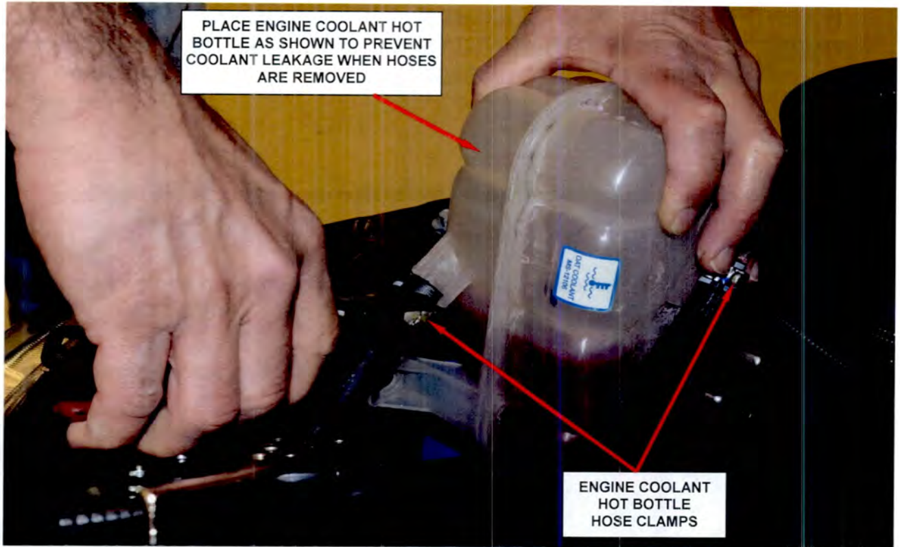
Figure 2 – Remove and Discard Hose Clamps
