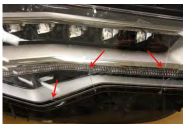
Figure 1. Cracks at bottom of headlight lens.
