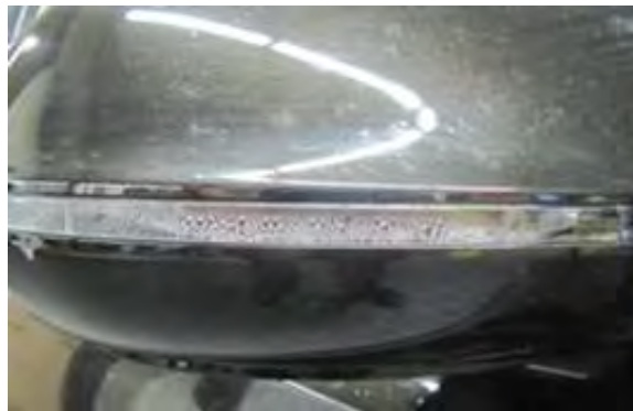
Figure 1 Condensation in turn signal lens
