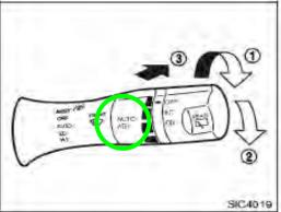
If a customer states the wipers do not work when the wiper lever is pushed down to the intermittent (INT) position, make sure the customer is familiar with the above information.
