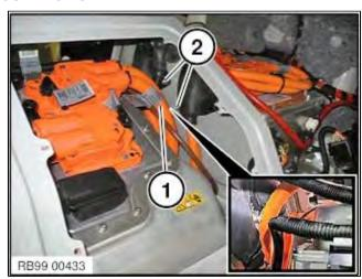
1. When reinstalling the EME/E-motor assembly after the greasing service, make sure that the HV cables (1) are not in contact with the M10 (2) nuts (approximately 1" of clearance is required) from the cable ducts on the right wheel housing.
