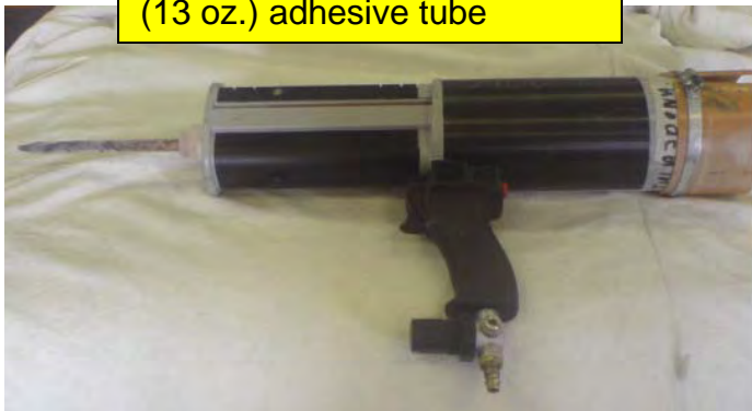
Plexus applicator with 380 ml (13 oz.) adhesive tube
