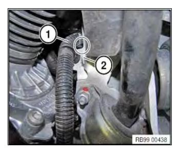
2. The correct distance (circled area) between the EPS harness (1) and the edge of sub-frame assembly (2) must be between 5 and 8 mm.
