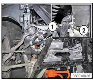
1. The EPS harness (1) must be positioned away from the subframe member (2).
