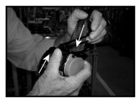
With the retractor in the normal installed position and the belt aligned straight out from the retractor, pull to extract the belt.
