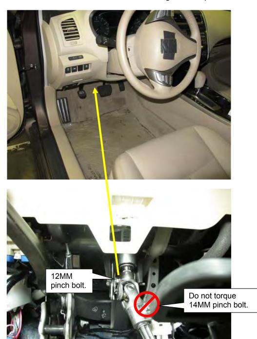
2. Torque 12MM pinch bolt to 18.5 ft-lb (25 NM).
