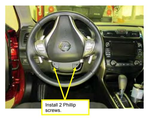
• Install 1 Phillip screw on bottom and to secure finisher to steering column.
