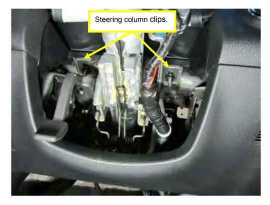
• Inspect to ensure clips are fully seated to bracket.
