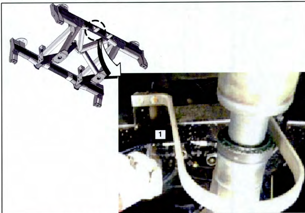
Figure 2. Rear of drive suspension support structure.
