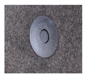
1. Align the upper piece of the mat retainer to the center of the retainer hole. Turn the mat over while maintaining the center position of the retainer.
