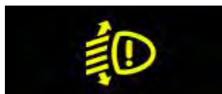
Figure 1. The dynamic headlight range control warning light.
