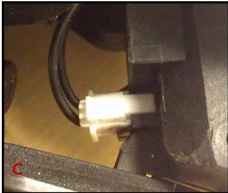
Figure 4. Connector "C" shown in the locked position.
