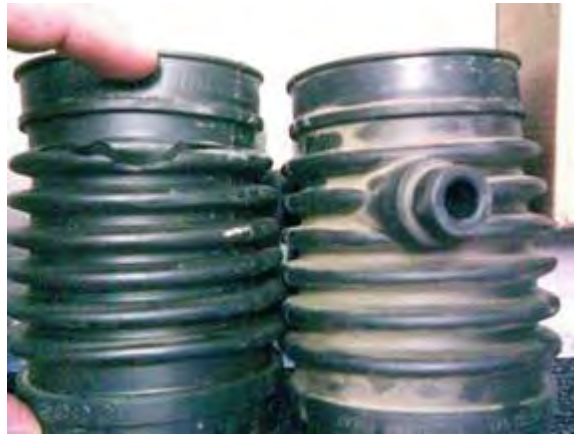
Figure 3. Crack in the intake hose.
