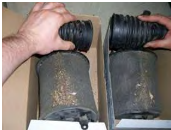
Figure 1. Example of excessive dirt on air filters.
