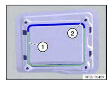
4. Smooth the ends of the butyl rope (1) to the sealing surface.
