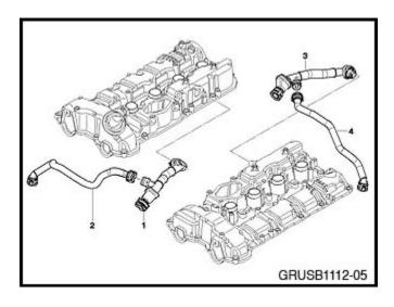
3. If the index number is "7" or lower, both crankcase ventilation connecting lines and vent pipes need to be replaced.
