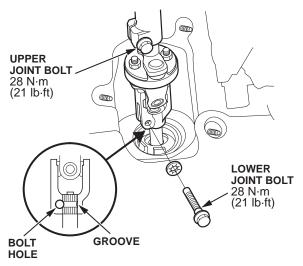
20. Pull on the steering joint to make sure it's fully seated, then tighten the lower joint bolt and the upper joint bolt to the torque in the illustration.
