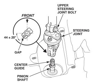
19. Align the bolt hole on the steering joint with the groove around the pinion shaft, then loosely install the lower joint bolt. Make sure the bolt is securely in the pinion shaft groove.
