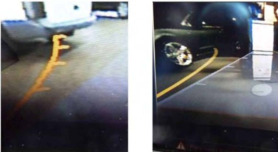
Figure 3. Guide lines of a vehicle without Peripheral View Camera (left) and guide lines of a vehicle with Peripheral View Camera (right).
