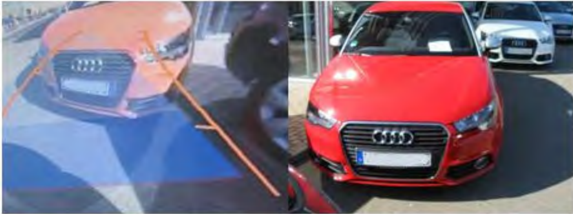
Figure 2: Camera image in MMI screen (left) and actual color of objects as seen by human eye (right).
