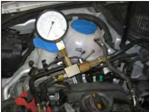
Figure 1. VAG 1318 gauge installed on a 2.0L TFSI.
