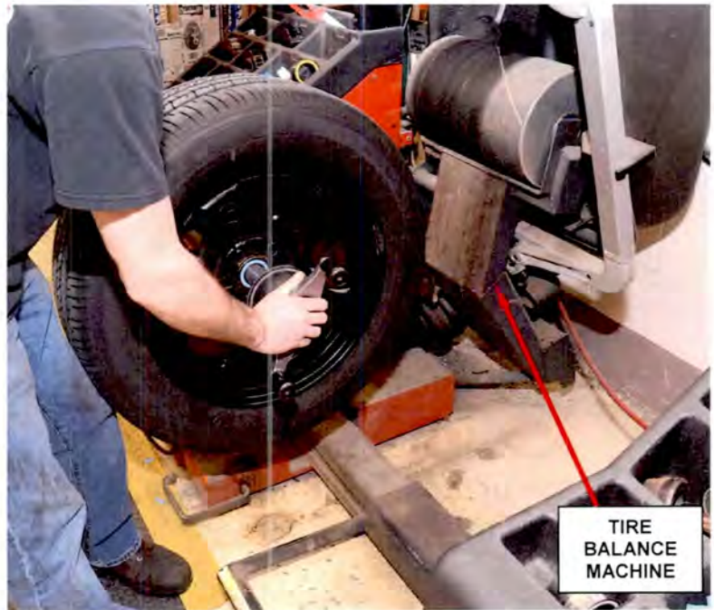
Figure 7 – Install Wheel/Tire on Balance Machine
