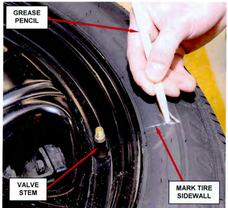
Figure 1 – Mark Tire Sidewall
