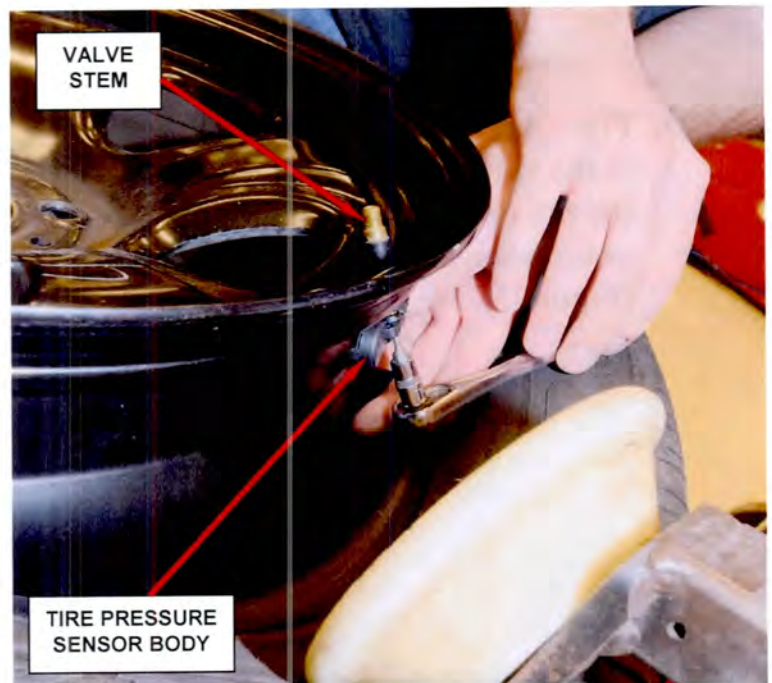
Figure 4 – Sensor Retaining Screw
