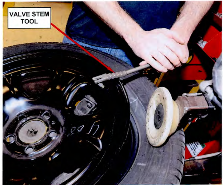
Figure 5 – Remove Old Valve Stem
