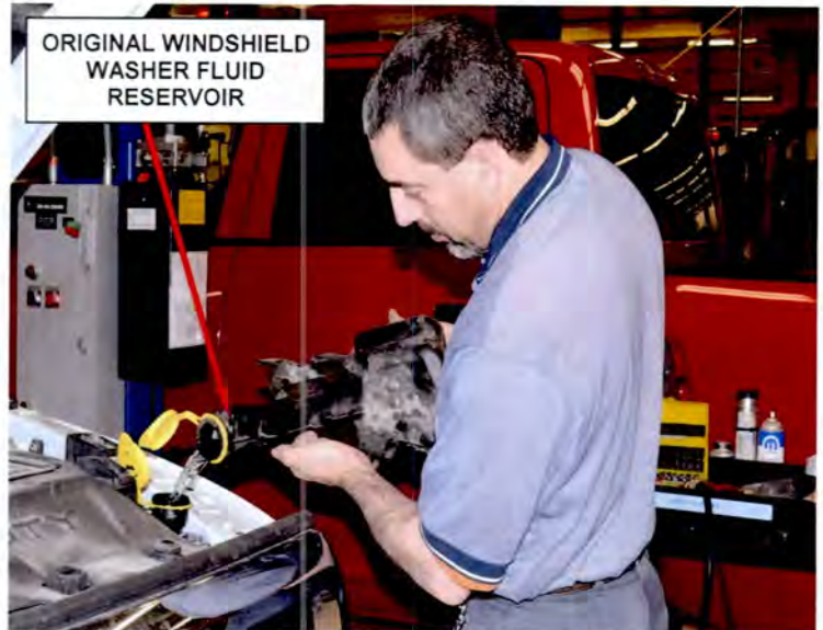
Figure 6 – Transfer Washer Fluid
