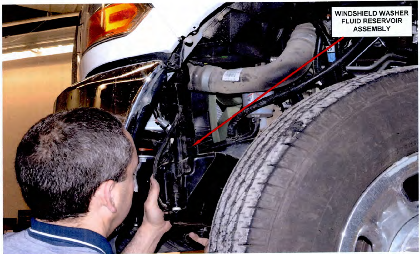
Figure 5 – Remove/Install Windshield Washer Fluid Reservoir Assembly
