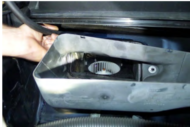
Figure 1. Applying water through a hose to check for water leaking into the fresh air intake.
