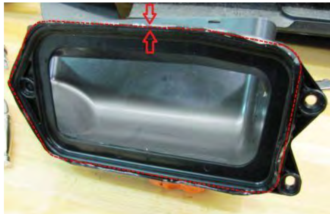
Figure 2. Location to apply the butyl cord is shown by arrows, and shown with the red dotted line.
