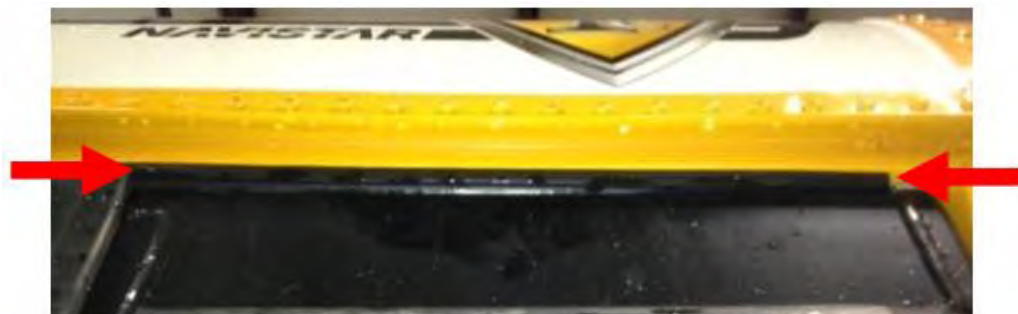
Upper Door Casing Seal Evenly Compressed
