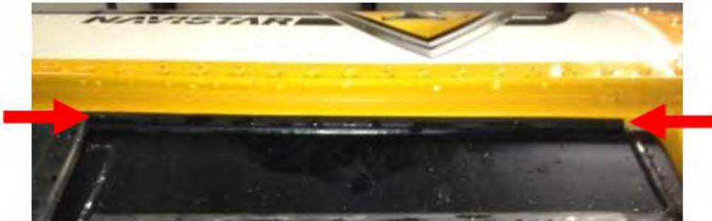
Upper Door Casing Seal Evenly Compressed
