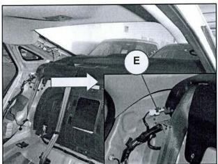
6. Remove the package trim (F) by unfastening five mounting screws and four fasteners.
