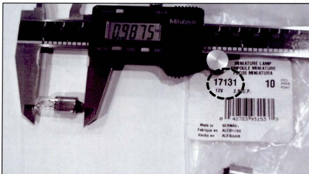
Figure 2. Correct bulb length ( just under one inch ).
