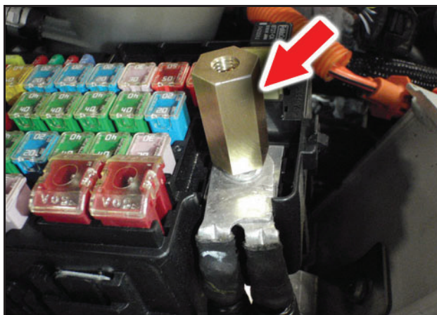
FST9001 - Battery Charging Terminal Adaptor (red arrow) installed on the B+ post in the PDC.
