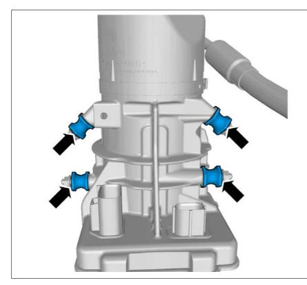
Check the condition of the rubber bushings. Replace them if damaged.
