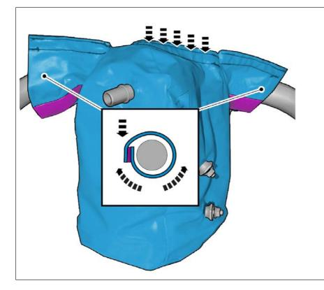
Continue installing the cover. Wrap it over the wiring harness and oil line as shown.
