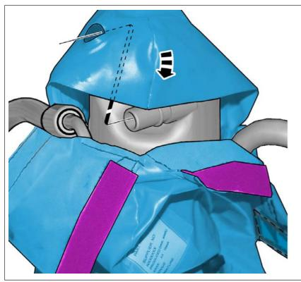
Install the top of the cover over the unit as shown.
