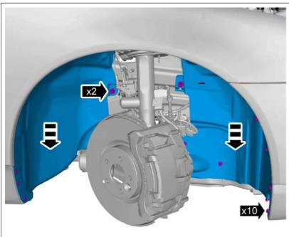
Remove the inner wheel housing as shown.
