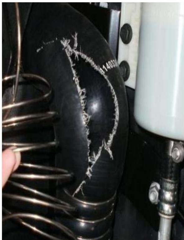
Figure 1 Burst CAC Hose
