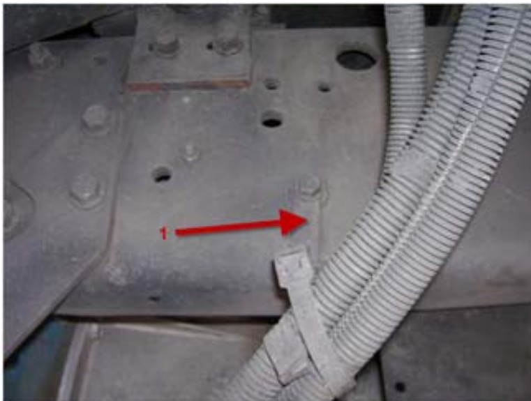
Figure 6 Routing and Clipping Points to be Aware of on an I6-Equipped Unit
