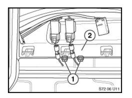
8. Install the new cable tie with holder (1) (P/N 61 13 0 302 824) and fit to the carrier (2). Remove the cable tie for later use.
