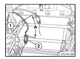
11. Locate the yellow side airbag connector (2). Cut the wire as shown, 100mm from the connector (A).
