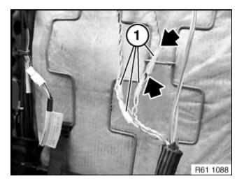
40. Slide the shrink tubing (1) over the crimp connections and heat up using a hot air blower until glue escapes onto the triggering circuit wires, indicated by arrows.
