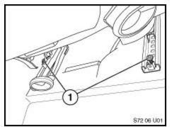
3. Remove the (4) mounting screws from the front seat with the stored fault.
