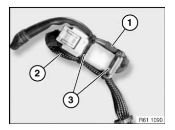
sections (1) and (2) at the connection to form an "S" shape. Secure with cable ties (3) (P/N 61 13 0 141 326). Take care to note the position of the cable fasteners. **Do not use Stabilant 22 or any other contact enhancer on the connections.**
