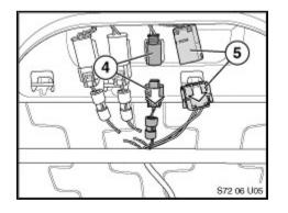
Disconnect the remaining connectors (4) and (5), and remove the seat from the vehicle. Connector (4) may not be on all vehicles.
