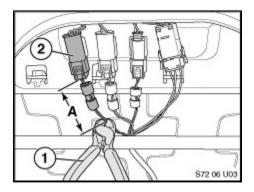
5. Locate the yellow side airbag connector (DO NOT DISCONNECT).
