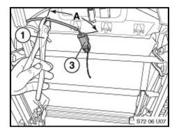
12. Locate the blue seat tensioner connector (3). Cut the wire as shown, **100mm from the connector** (A).
