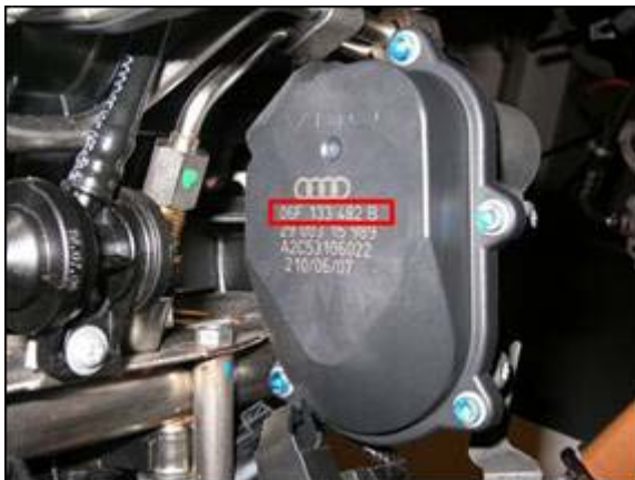
Figure 1. Part Number Location on The Intake Flap Motor V157. P/N 06F 133 482 E should be installed.
