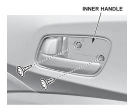
Remove the pull pocket mat, then remove the screw.
