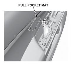
6. Starting at the bottom edge of the door panel, detach the clips with a commercially available trim pad remover.
