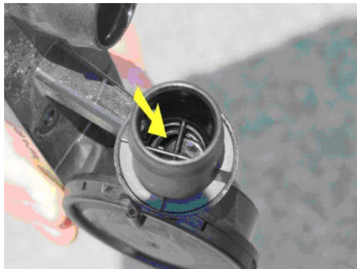
Figure 2. The guide pin of the check valve in the intake manifold side of the valve. (Depending on part number, the check valve may be installed horizontally inside the housing.)
