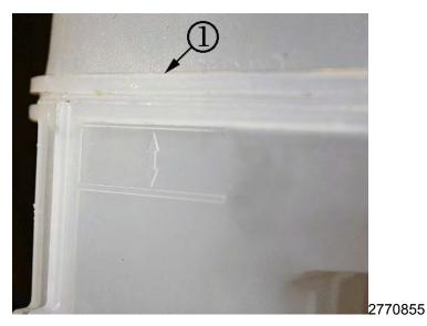
29. Re-check coolant level. Ensure the coolant level is to the top of the tank seam (1).
