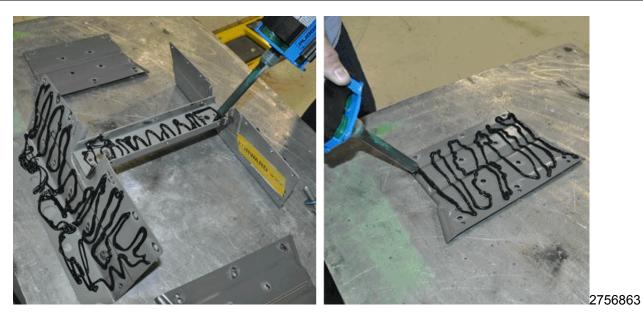
**Caution:** Ensure the Pliogrip two-part polyurethane mix is uniform in color BEFORE applying it to the parts. Discard the first 25 mm (1 in) of the mix that is not uniform. The color of the polyurethane varies. The illustrations in this bulletin show the polyurethane mix in black or green. The Pliogrip two-part polyurethane has a 30-minute open time. The application of the Pliogrip two-part polyurethane and the assembly of the reinforcement assembly must be completed in 30 minutes.
