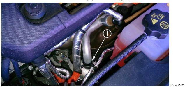
10.16 Install new harness clip (1) (from the kit) on the A/C line above existing harness clip on the ACCM high voltage pigtail.
