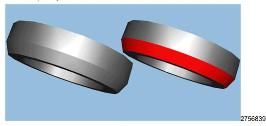
**Note:** Butyl should <u>only</u> be applied in the chamfer (red face) of the crush limiter. Refer to illustration. Butyl should not be present in the metal-to-metal joint between RESS cover, reinforcement plate and longitudinal rails.
