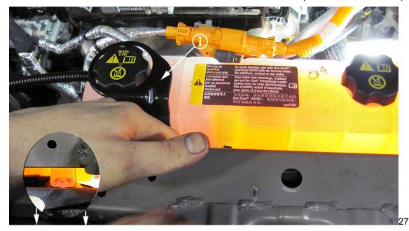
30. Install locking bracket (1) on vehicle right side reservoir securing the bracket and the reservoir with the bolt provided in the kit. Tighten bolt from front side of tie bar.
