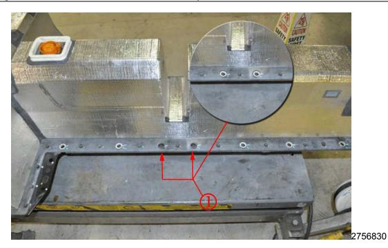
**Note**: The aluminum crush limiters are chamfered and must be installed with chamfer side down.
