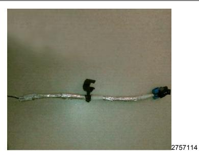
10.7 Locate the coolant level sensor jumper from service kit 19260759 and strip 13 mm (1/2 in) of insulation from the two wire ends.
