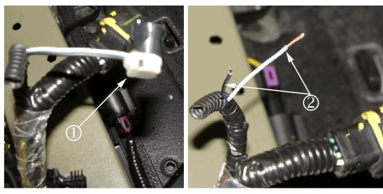
10.6 Cut off the wires at the back of the refrigerant temperature sensor (1) connector and strip 13 mm (1/2 in) of insulation from the two wire ends (2).
