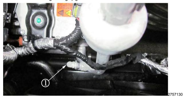
10.17 Put a dime-sized dab of RTV, P/N 88861417 (or equivalent) over exposed refrigerant temperature sensor (1) to cover exposed terminals.
