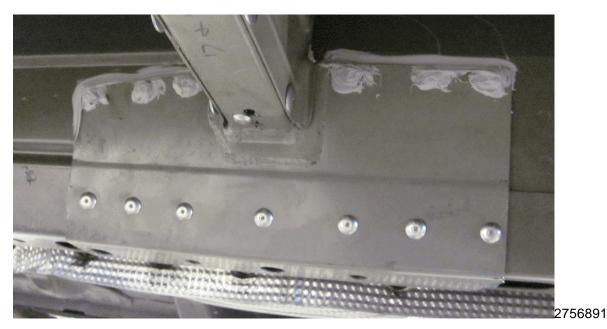
27. Apply RTV, P/N 88864346 (or equivalent), on and around each of the six upper rivet heads along each side of the reinforcement assembly. The other rivet head locations do not require sealer.
