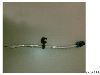
10.7 Locate the coolant level sensor jumper from service kit 19260759 and strip 13 mm (1/2 in) of insulation from the two wire ends.
