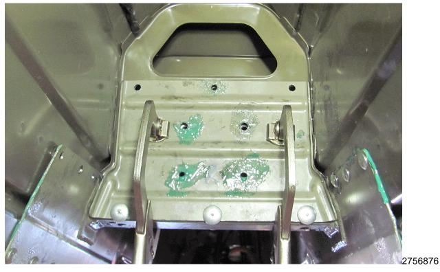
**Caution:** To ensure the pop rivets are installed correctly, use two hand clamps or "C" clamps to hold the plates into position. Make sure the rear plate is pressed against the vehicle body in each location as each rivet is being installed.
