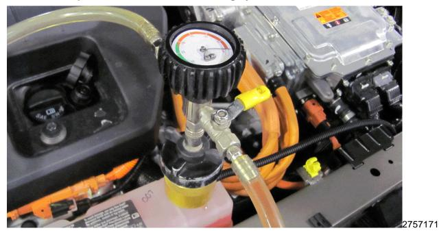
17.1 Use the VAC-N-FILL equipment without the 152 mm (6 in) hose extension.
