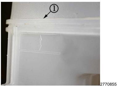
29. Re-check coolant level. Ensure the coolant level is to the top of the tank seam (1).
