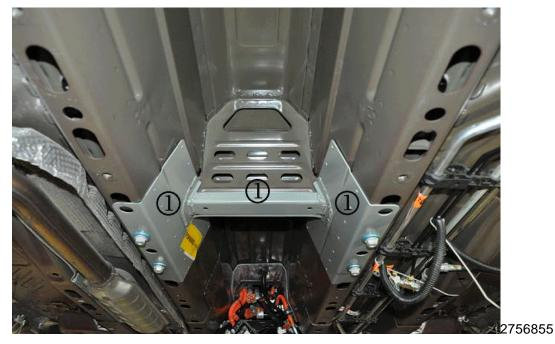
7. Attach the reinforcement assembly (1) to the car body using the four shorter M10 bolts from the kit. Tighten bolts to 25 Nm (19 lb-ft). Make sure the reinforcement assembly is centered from side to side within the tunnel of the vehicle body.
