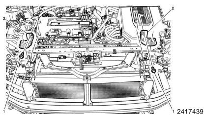
25. Reinstall radiator mounts (2). Tighten bolts to 22 Nm (16 lb-ft).
