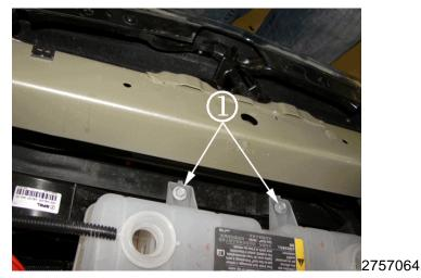
**Caution:** Do NOT use a prybar or similar tool to move the radiator module rearward, or damage to the radiator module can result.
