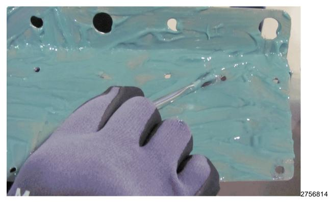
19. Coat drill holes and exposed metal with Pliogrip, P/N 7770B220, two-part polyurethane using a brush as shown in illustration.
