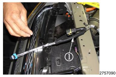
10.10 Install the new corrugated tube (1) that is provided in the service kit over the harness splice. The corrugated tube should overlap existing harness corrugated tube on both sides.
