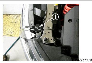
3. Remove windshield washer filler tube (1) by pulling up on it.
