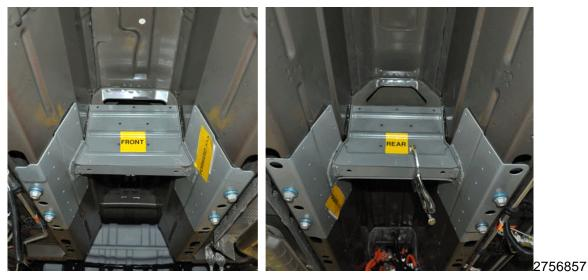
8. Locate the front and rear plates to the car body and hold in position using two hand clamps or "C" clamps. Make sure the front and rear plates are centered from side to side on the tunnel reinforcement of the vehicle body.
