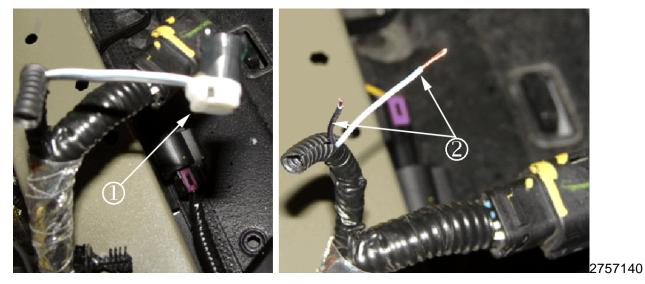
10.6 Cut off the wires at the back of the refrigerant temperature sensor (1) connector and strip 13 mm (1/2 in) of insulation from the two wire ends (2).
