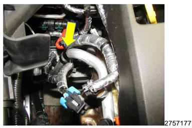
10.16 Install new harness clip (from the kit) on the A/C line above existing harness clip.
