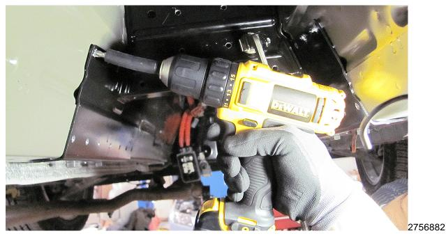
**Caution:** To avoid vehicle damage, place a drill stop on drill bits to ensure drill does NOT enter the vehicle beyond 19 mm (<sup>3</sup>/<sub>4</sub> in) in depth.
