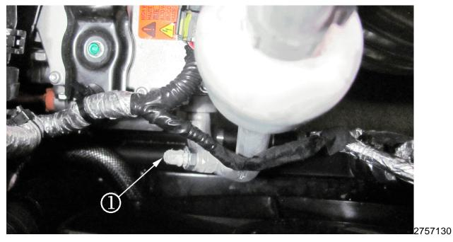
10.17 Put a dime-sized dab of RTV, P/N 88864346, (or equivalent) over exposed refrigerant temperature sensor (1) to cover exposed terminals.
