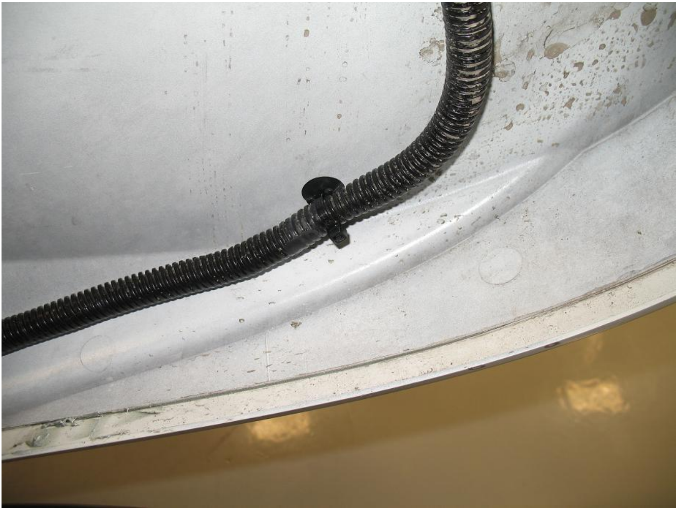
Figure 4 - Headlamp wiring harness (hood side) secured with P/N 3613346C91, combination retainer and wire tie
