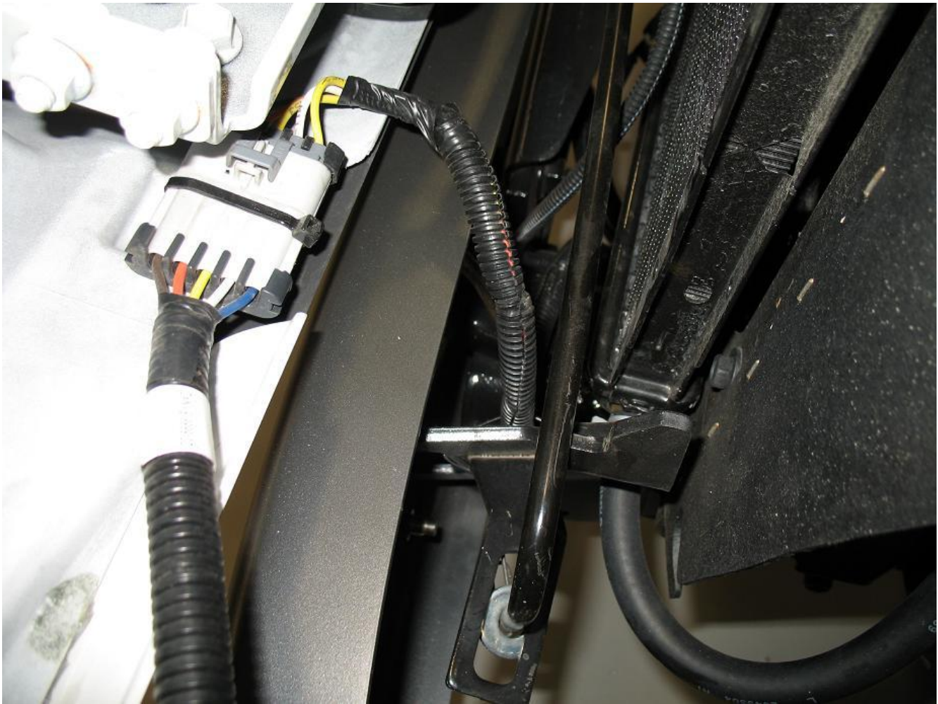
Figure 2 - Headlamp wiring harness (chassis side) in "as-built" location - note pinch point on harness
