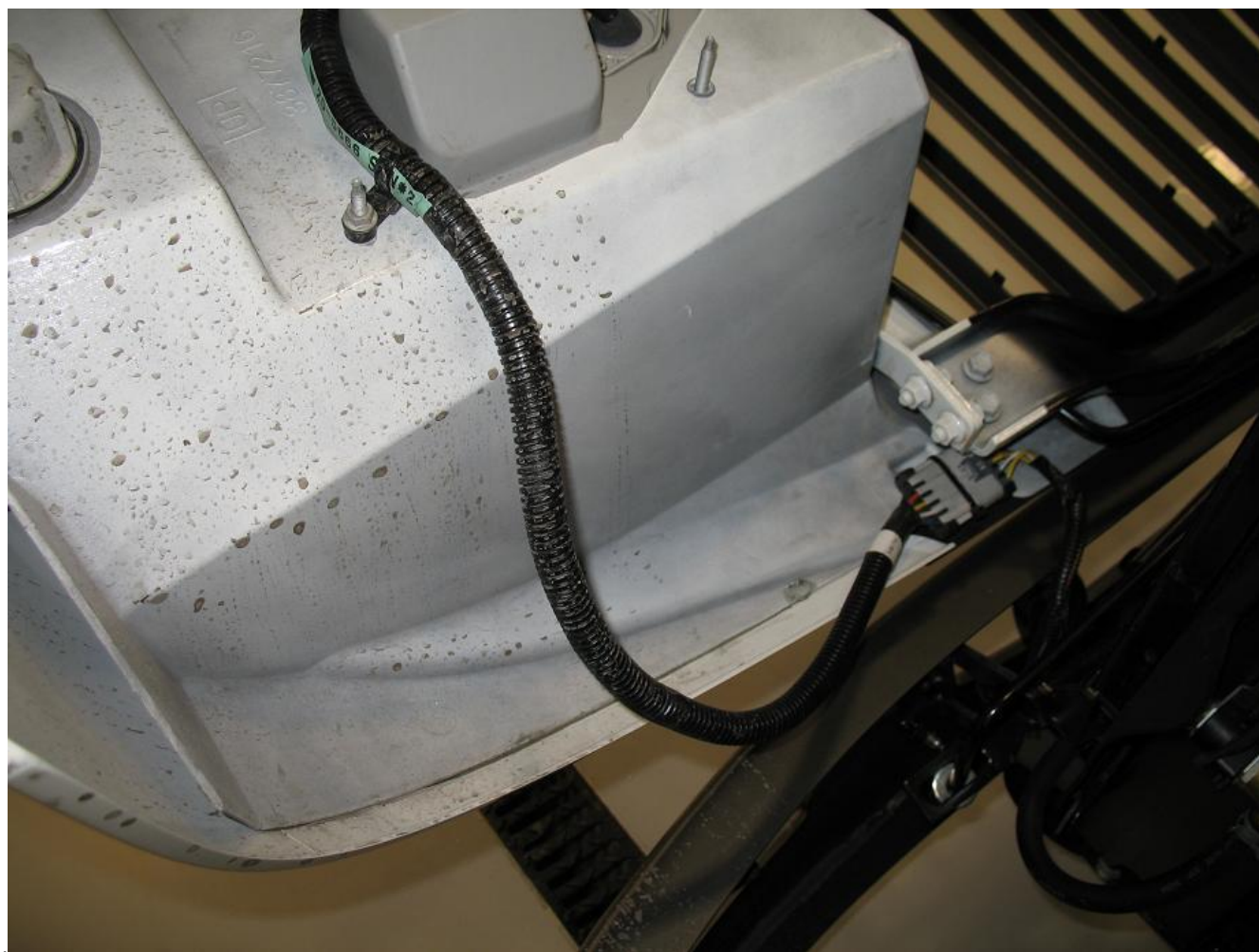
Figure 1 - Headlamp Harness in As-Built Configuration (note that connector may not be secured during assembly)
