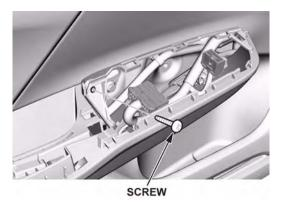
5. Carefully release the eight clips holding the door panel in place, and remove the panel by pulling upward.
