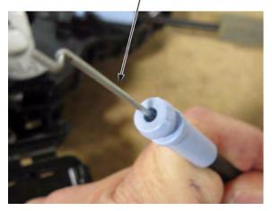
9. Apply DC 111 lubricant to the lock cable as shown.
