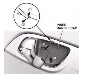
3. Remove the screw, then pull the inner door handle out of the door panel.
