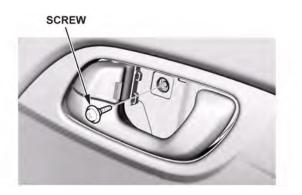
4. Remove the screw under the door handle.
