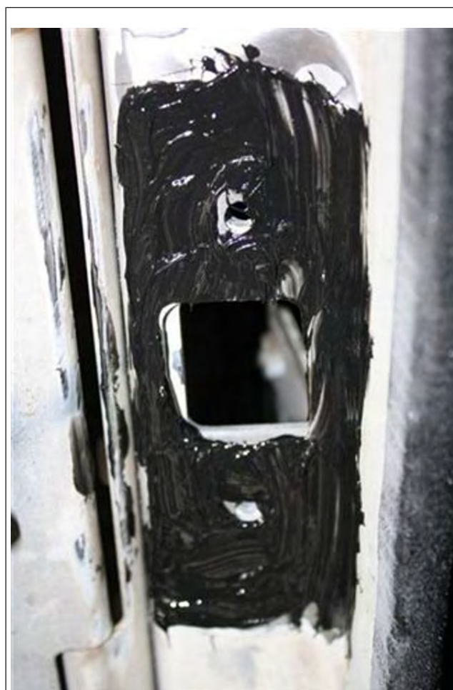
Fig. 5, Applying Urethane Adhesive
