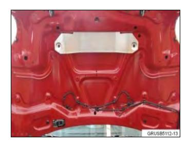
the heat shield notches line up properly, the shield will slide into the air grill completely. The two open holes in the bonnet will then align with the shield, allowing you to insert the two push-pins.
